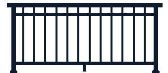
Mid-Rail Baluster Railing
